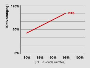
Below is a graph applied to the GRECALE and BOREA series that, with the same ventilation and number of tubes in the coil, due to the effect of different geometries and types of fins, express different drying levels to maintain the same real heat exchange performances in the cold room.
